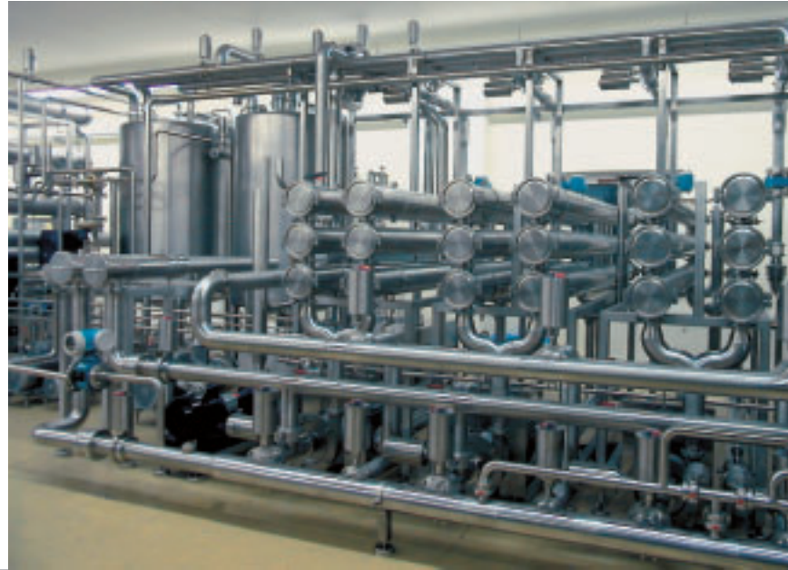
4-stage fully automatic UF-DF-RO-plant for the food industry
