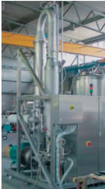
Fully automatic microfiltration plant for skimmed milk during functional testing in our workshop Dresden
