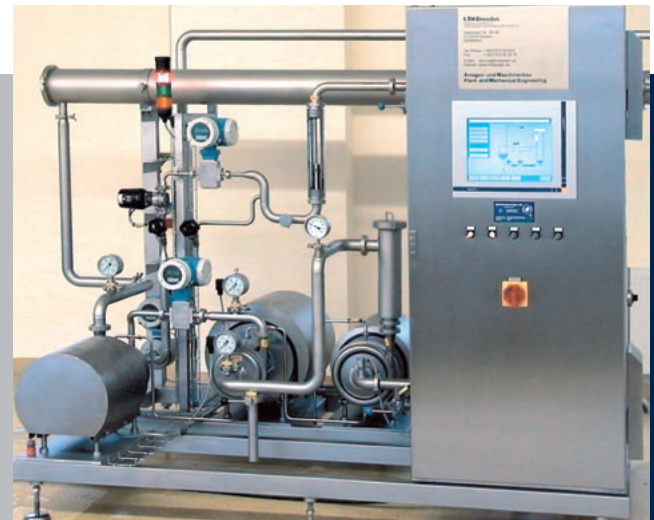
Pilotanlage Ultra-/Nanofiltration/Umkehrosnose Pilot plant Ultra-/Nanofiltration/Reverse Osmosis
